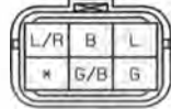
K-10 POWER DOOR LOCK ACTUATOR LH AND DOOR LOCK LINK SWITCH (DR1)
